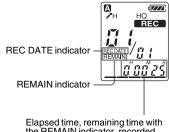
the REMAIN indicator, recorded date with the REC DATE indicator\*, or recorded time with the REC DATE indicator\*\*
